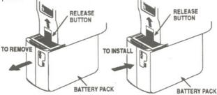
**Recharging the Nickel-Cadmium Battery Pack**
